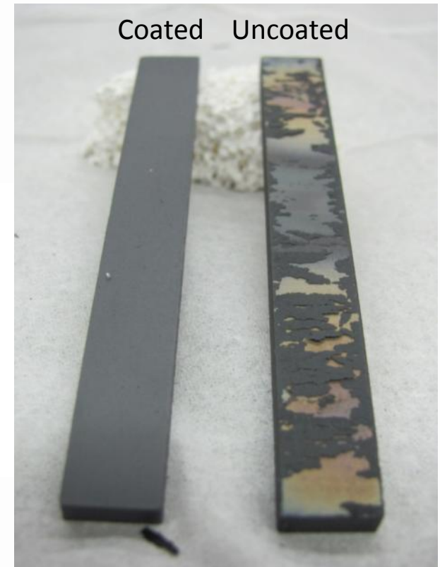
10 \mu\text{m} MCO coating on AL 441-HP substrate 900 °C, 200 hours, Air
