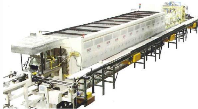
Controlled Atmosphere Electric Pusher Kiln
